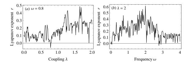
FIG. 6: (a) The Lyapunov exponent of the atomic walking versus coupling intensity  $\lambda$  with  $\omega = 0.8$ . (b) The Lyapunov exponent versus modulation frequency  $\omega$  with  $\lambda = 2$ . The initial atomic position is x(0) = 0, momentum p(0) = 0.4.
