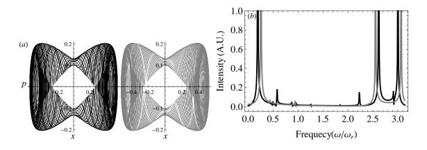
FIG. 7: (a)The phase portrait of a strict solution of Eq. (7) (left black orbit) and the Mathieu solution of Eq. (16) (right gray orbit) with parameters  $\lambda = 1$ ,  $\omega = 2.8$  and the initial position and momentum being x(0) = 0.2, p(0) = 0.18. (b) The corresponding power spectrum of the atomic momentum for the strict solution (black line) and the Mathieu solution (gray line).
