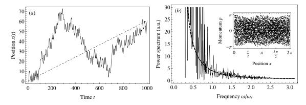
FIG. 5: (a) A typical random walking of a cold atom in a varying standing field of  $\omega = 0.8$ ,  $\lambda = 2$  with x(0) = 0, p(0) = 0.4. The dashed line is the average motion of the atom. (b) The corresponding power spectrum of the random walking (solid) and the average motion (dashed). The inset picture is the pase-space distribution of the walking mapped to  $[0, 2\pi]$ .
